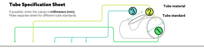
Run TubeRun tube wallBranch tubeBranch tubeBranch tubeBranch tubeO.D. (1)thickness (2)O.D. (3)O.D. (3)O.D. (3)O.D. (3)O.D. (3)
