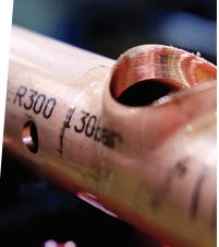
**T-DRILL S-56 PC**, is a cutting-edge punching and collaring unit that combines two methods in a single unit, ensuring unparalleled efficiency and precision.
