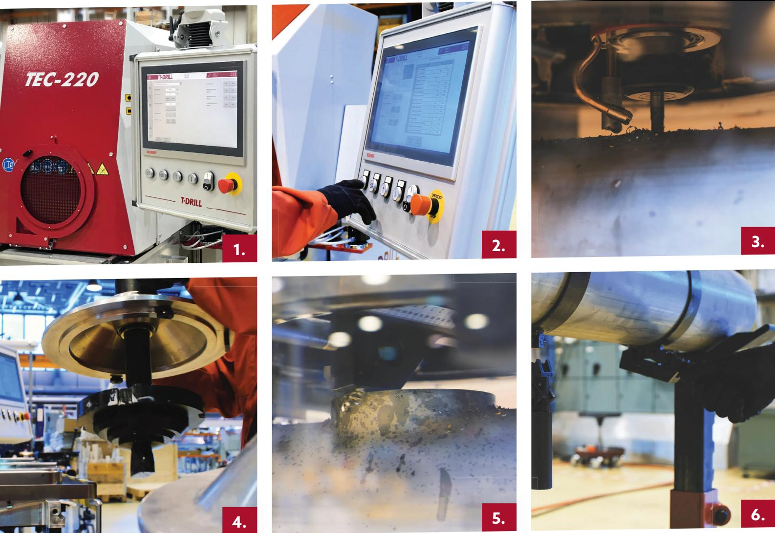
1. The user-friendly 15" operation panel is used for controlling work cycle operations. It also enables manual drive mode and service pages.
